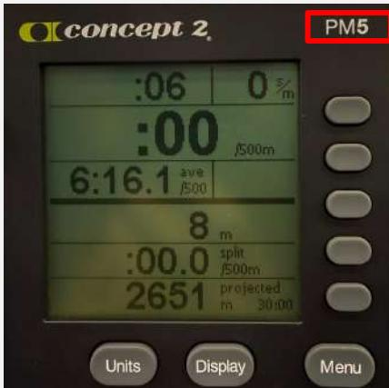
Press the Menu button at the bottom right of the monitor.
